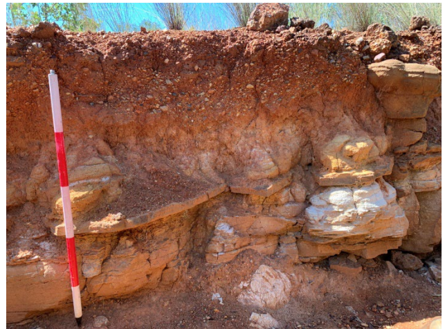
Plate 9: Soil section that has been quarried for agricultural use. The section shows the soil profile of the south-western hill crest within the Activity Area. The section shows soil that is consistent with those found on lower hill slopes and flats in Activity Area. From base, profile shows brittle sandstone sediment with a thin layer of basalt material. Sandstone, clay/silt layer, red soil with alluvial pebbles, eroding sandstone and large conglomerate ironstone pieces with quartz inclusions.
